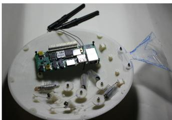
The first prototype of robot fish with SMA-actuated fin for pitch control (BSLab, 2012) and current design based on piezoelectric actuators.
