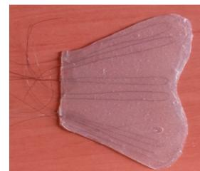
SMA-actuated flexible tail fin for roll control (BSLab, 2014)
